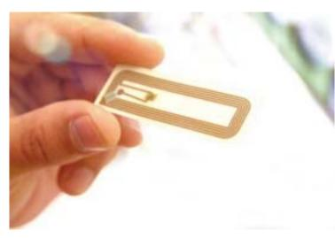
The RFID device serves the same purpose as a bar code or a magnetic strip on the back of a credit card or ATM card; it provides a unique identifier for that object. And, just as a bar code or magnetic strip must be scanned to get the information, the RFID device must be scanned to retrieve the identifying information.
